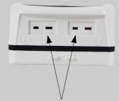
Connectors for thermocouple probes
